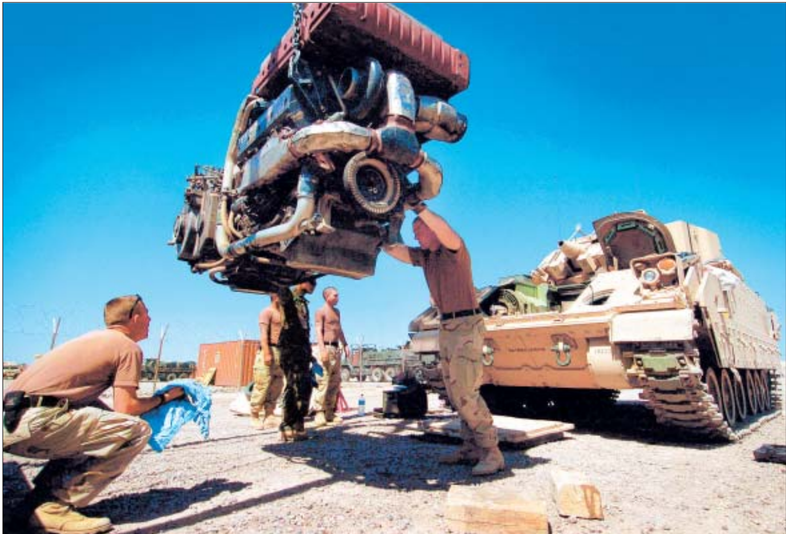
Sgt. Erik Houghton, left, examines the engine of a Bradley Fighting Vehicle that broke down with an oil leak. Up to 5,200 Fort Carson-based troops in the 3rd Armored Cavalry are on their second Iraq tour; they say their work is difficult and dangerous, but it beats sitting around.
